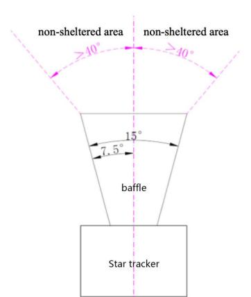
Be sure: Nothing sheltered in the field of view: the circular cone of  $80^{\circ}$  around the top of the Baffle.
