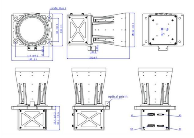
Note: This sketch should include body size, mounting size, mounting plane, mounting point (aperture and its tolerances, center distance and its tolerances), position tolerances for guide pins and holes, direction, location, type and number of electrical connectors, the operating hole, the lap (position and length), the registration measurement reference for calibration and testing.
