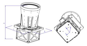
Note: The origin of the coordinates lies in the geometric center of the outer surface of the lower shell (see "Instrument diagram");
