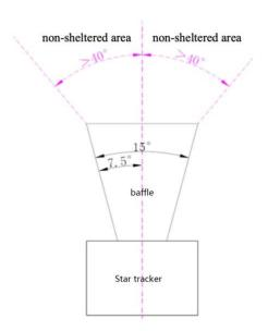
Be sure: Nothing sheltered in the field of view: the circular cone of  $80^{\circ}$  around the top of the Baffle.
