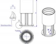
Note: The origin of the coordinates lies in the geometric center of the outer surface of the lower shell (see "Instrument diagram");
